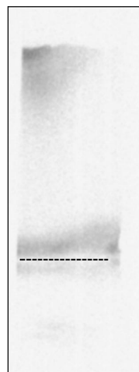
FIG. 7. EUV pinhole image of the discharge at 40 ns before the pinch, recorded at an increased MCP voltage of 6.24 kV. The area of the image corresponds to an area of 1.6 mm wide and 4.2 mm high in the source. The dashed line gives an indication of the position of the surface of the cathode. Like in the visible light images, the real anode position corresponds to the top of the frame, but the region closest to the anode is obstructed from the view. In this image, some EUV emission is visible from the region just outside this obstruction.
