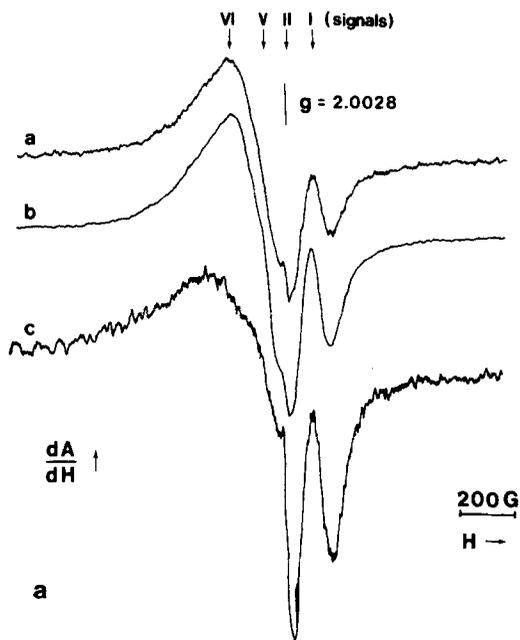
FIG. 2a. ESR spectra of promoted molybdenum-on-alumina catalysts (recorded at 20 K): (a) Ni(2.7)-Mo(10.5)/ $\gamma$ -Al<sub>2</sub>O<sub>3</sub>, sulfidic route,  $R.G.$  =  $2 \times 10^3$ ; (b) Ni(4)-Mo(12)/ $\gamma$ -Al<sub>2</sub>O<sub>3</sub> (C), oxidic route,  $R.G.$  =  $5 \times 10^2$ ; (c) Co(2.7)-Mo(10.5)/ $\gamma$ -Al<sub>2</sub>O<sub>3</sub>, sulfidic route,  $R.G.$  =  $4 \times 10^3$ .
