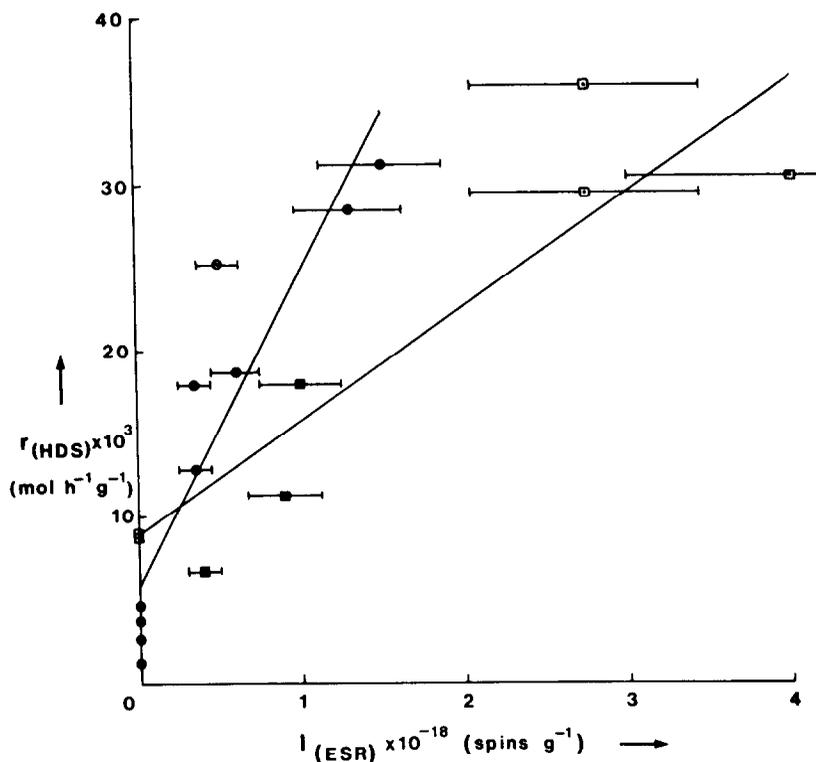
FIG. 3. Thiophene reaction rate versus ESR signal VI intensity for molybdenum-containing catalysts (□, conventionally prepared; ■, sulfidic route), and for tungsten-containing catalysts (○, conventionally prepared; ●, sulfidic route).
