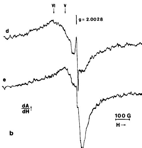
FIG. 2b. ESR spectra of promoted molybdenum-on-silica catalysts (recorded at 20 K): (d) Ni(2.7)-Mo(10.5)/SiO<sub>2</sub>, sulfidic route,  $R.G.$  =  $8 \times 10^3$ ; (e) Co(2.7)-Mo(10.5)/SiO<sub>2</sub>, sulfidic route,  $R.G.$  =  $4 \times 10^3$ .
