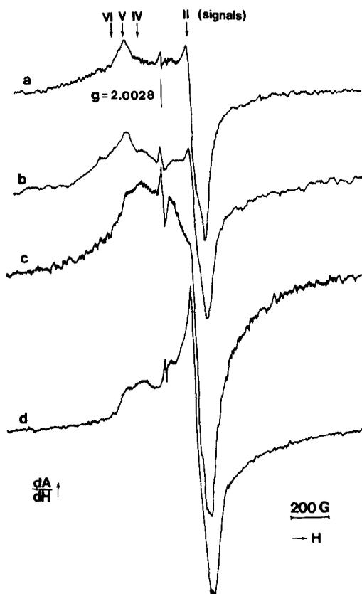
FIG. 1. ESR spectra of unpromoted tungsten catalysts (recorded at 20 K): (a) W(17.6)/SiO<sub>2</sub>, sulfidic route, receiver gain ( $R.G.$ ) =  $2 \times 10^3$ ; (b) W(19.3)/SiO<sub>2</sub> (C), oxidic route,  $R.G.$  =  $5 \times 10^3$ ; (c) W(17.6)/ $\gamma$ -Al<sub>2</sub>O<sub>3</sub>, sulfidic route,  $R.G.$  =  $4 \times 10^3$ ; (d) W(19.3)/ $\gamma$ -Al<sub>2</sub>O<sub>3</sub> (C), oxidic route,  $R.G.$  =  $1 \times 10^3$ .
