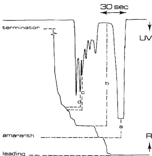
Fig. 1. Anionic separation of uremic serum ultrafiltrate (0.5  $\mu$ l injected) by isotachopheresis (test run). UV absorption and conductivity detector traces are shown (R = resistance). a = Amaranth red; b = phosphate; c = hippurate; d = urate. Conditions are given in Table I.
