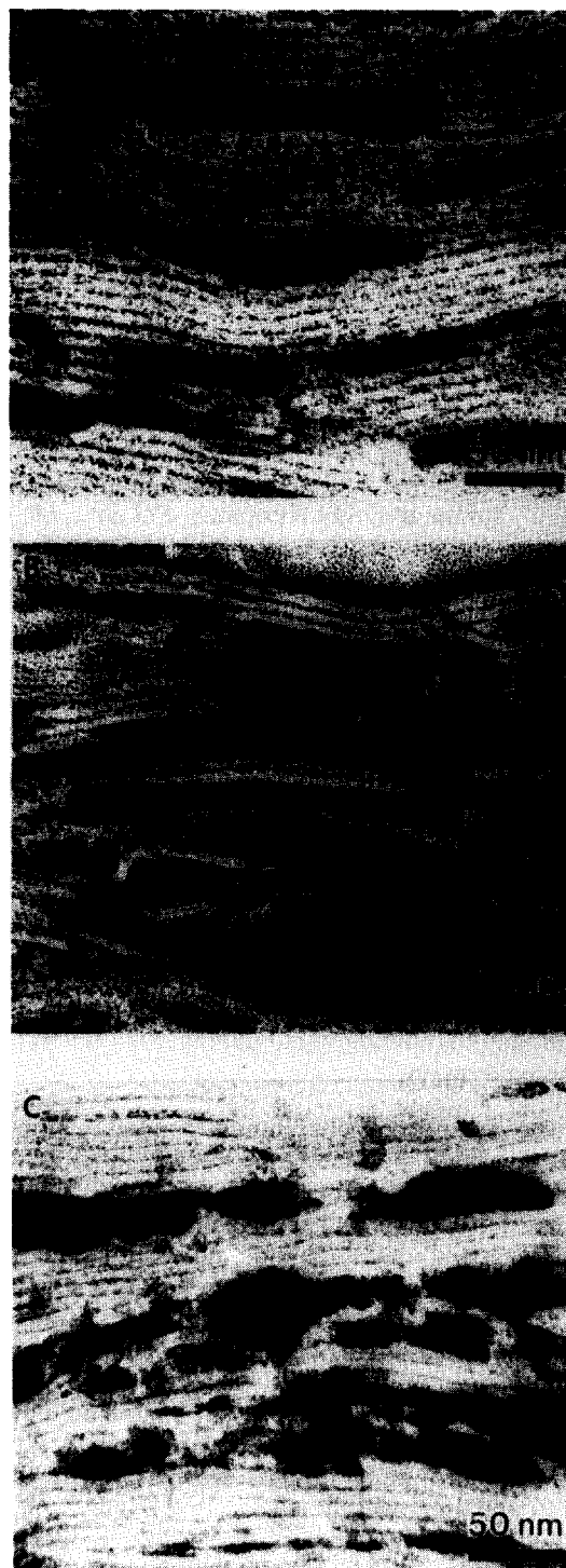
Figure 1 Transmission electron micrographs of solution-crystallized UHMW-PE/ t -1,4-PB films. t -1,4-PB content (wt%): (A) 10; (B) 20; (C) 50
