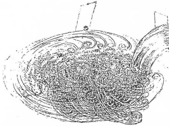
Figure 1.2. Early drawings of turbulence by Da Vinci, showing a pair of counter rotating vortices in the middle of a random wake [17].
