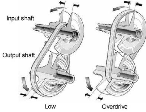
Fig. 1. Working principle of a Continuously Variable Transmission
