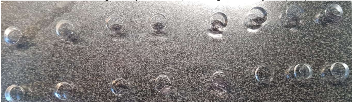
The result of using the paper clip with hot (left four) and already solidifying (right four) gel
