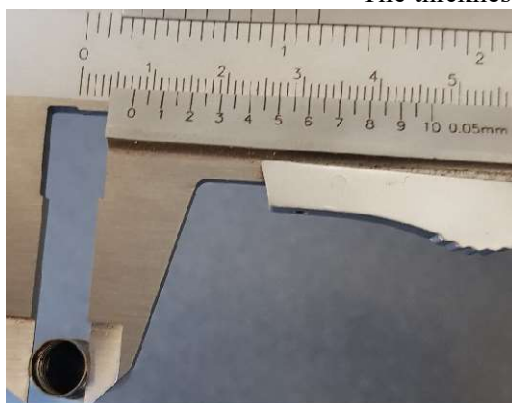
The hole (left) and pipette (right) diameter
