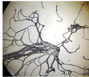
Figure 7.6: The result of SU8-on-NOA81 photolithography with acetate and HMDS treatment.
