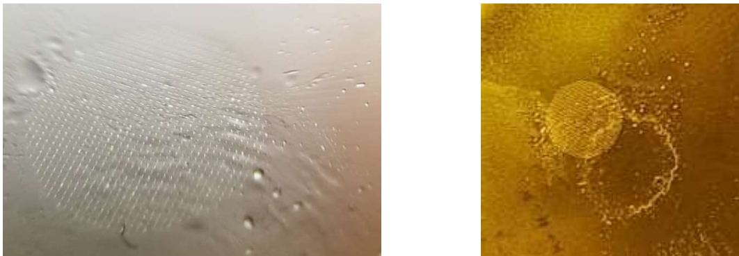
Figure 7.2: The result of SU8-on-NOA81 photolithography from under a microscope (left) and in a larger view (right). The waves seen in the microscopic picture are SU-8 ridges. These ridges appear to be concentric as observed in the larger view
