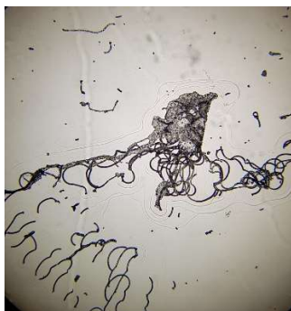
Figure 7.7: The result of SU8-on-NOA81 photolithography with a slow cooled PEB (left) and increased UV-light intensity (right).
