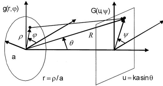
Fig. 1. Far-field  $G(u, \psi)$ , radiated by a circular aperture with radius  $a$ , excited by a general source  $g(r, \varphi)$ .
