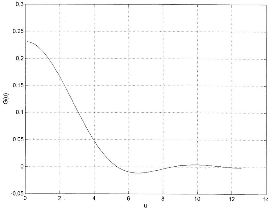
Fig. 3. Radiation pattern  $G(u)$  of a circular aperture with a source excitation, shown in Fig. 2, calculated by TSE method.
