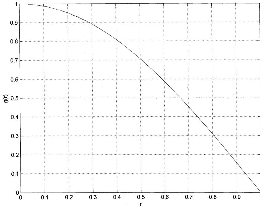
Fig. 2. Source excitation of a circular aperture with radius  $a = 2\lambda$ :  $g(r) = \cos(\delta r)$ ,  $\delta = \pi/2$ .
