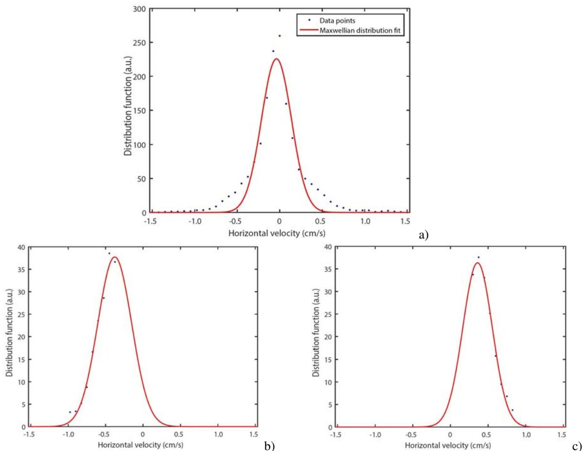
**Fig. 4** Dust particle distribution functions for velocity horizontal projections on side view of dust structure on Fig. 2 (dots — experimental data, line — Maxwell distribution): a) total velocity distribution, b) velocity distribution for particles with negative velocities (moving to the left), c) velocity distribution for particles with positive velocities (moving to the right).
