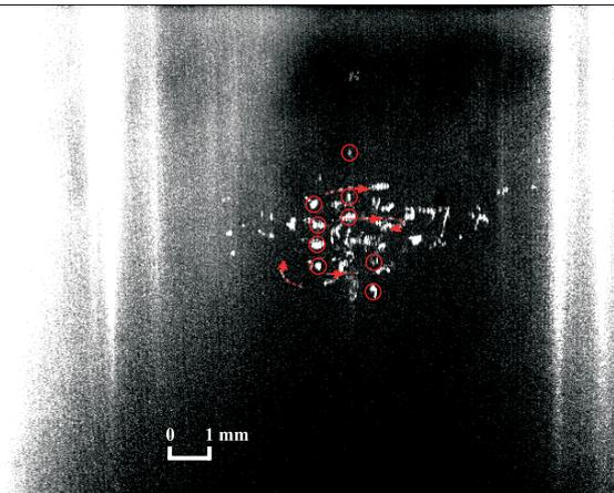
**Fig. 3** Side view of typical two-component dust structure in dc discharge striation at 77 K (gas pressure 0.3 Torr, discharge current 1.1 mA). The image is the result of superposition of 13 consequent frames. Circles indicate some particles in dust chains, arrows indicate the movement of some orbiting particles.
