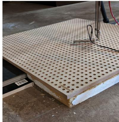
Figure 2 – Placement of the PU probe above one of the systems characterized (perforated facing II backed with porous material).
