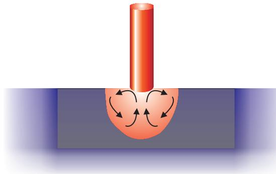
Figure 5: Convection in the melted region.
