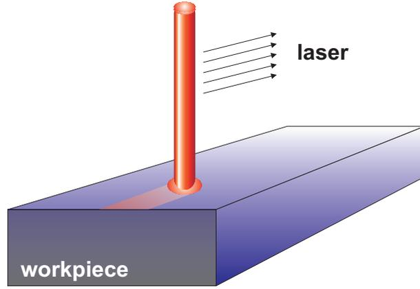
Figure 1: Laser surface remelting.
