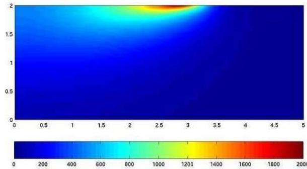
Figure 3: Temperature profile after 60 time steps calculated on a composite grid.
