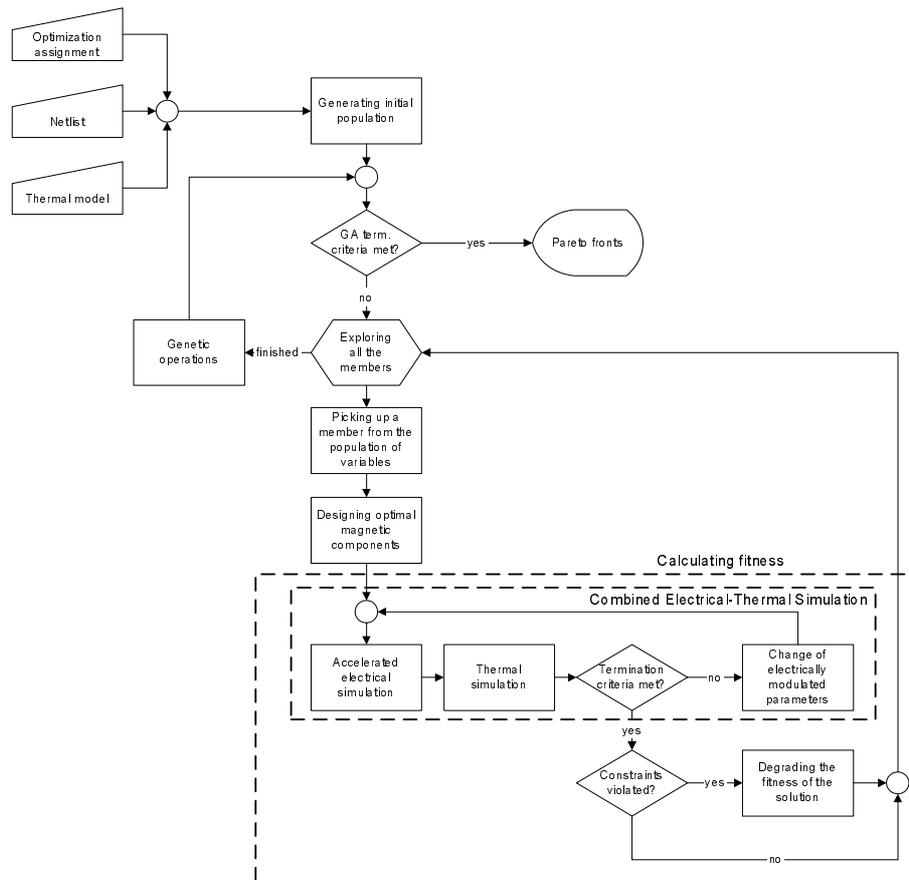
Figure 1: Converter optimization flowchart
