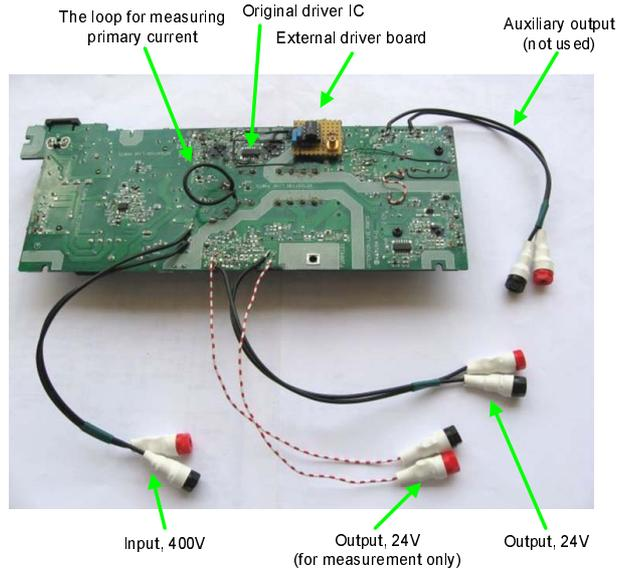
Figure 6: Modified converter board
