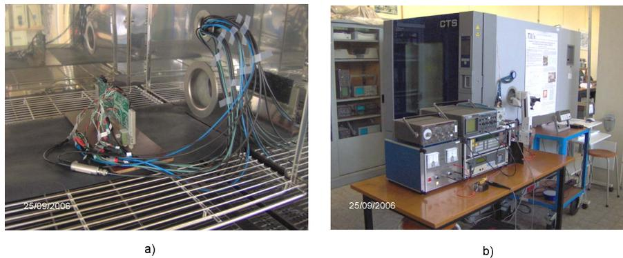
Figure 4: A setup for experimental identification of the thermal model: a) General view of the setup b) Converter under investigation
