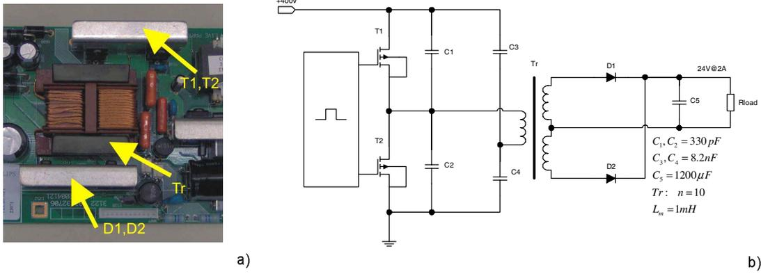
Figure 2: LLC converter : a) Photograph b) Schematic diagram
