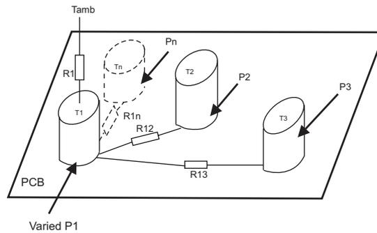
Figure 3: Experimental method for deriving the thermal model
