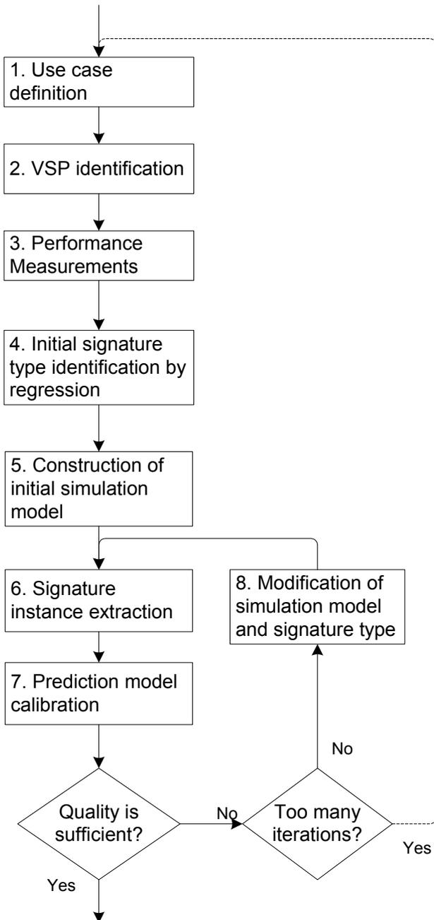
**Figure 2. Construction of simulation and prediction models**
