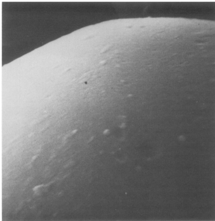
FIG. 2. SEM of glass sample 5 (hydrophilic). Horizontal side: 10 \mu\text{m}
