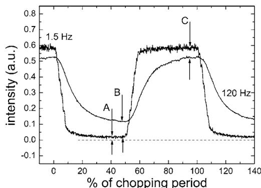
Fig. 3. Comparison of the QMS signals at 1.5 and 120 Hz chopping frequency measured with argon gas in the vacuum chamber. The  $x$  axis scale is in % of the chopping cycle. The increase of the background signal at high chopping frequency is clearly visible when A and B are compared. The difference between B and C indicates that chopper influences the conductivity in the second stage. The time delay of 0.8 ms observed on the signal is the artifact of the analog output of the HIDEN instrument.
