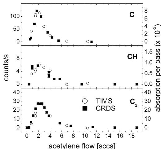
FIG. 9. C, CH, and  $C_2$  radical measurements as function of acetylene gas flow into the reactor. The arc current of 48 A and argon gas flow of 100 sccs is used. The TIMS results are compared with CRDS absorption measurement of these radicals performed in the past under the same conditions.
