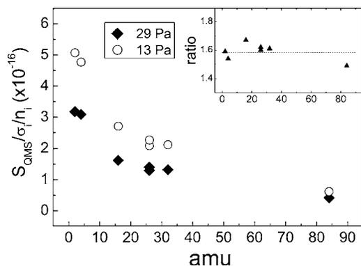
FIG. 5. QMS signals of  $\text{H}_2$ , He,  $\text{CH}_4$ ,  $\text{C}_2\text{H}_2$ ,  $\text{O}_2$ , and Kr, divided by their electron impact ionization cross section and their vessel density, at two different pressures of 29 and 13 Pa. Argon is used as a dilution gas. Insert shows the ratio of the signals.
