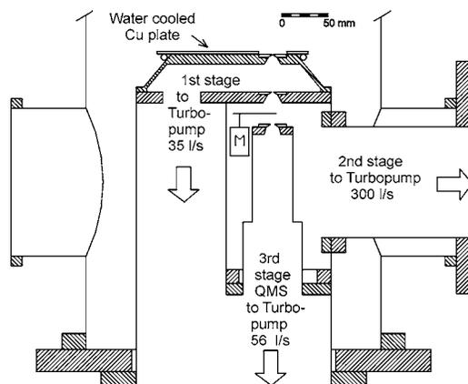
FIG. 2. Detail of the threshold ionization mass spectrometer housing. The beam chopper is drawn only schematically.
