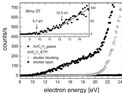
FIG. 12. QMS signal at  $m/e$  ratio of 37 as function of electron energy. Vessel pressure 29 Pa, arc current 48 A, ring-substrate distance 25 cm, and  $C_2H_2$  flow 18 sccs. Electron energy scale enlarged to show 12.3 eV change of slope.
