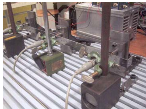
Figure 5. Flexible beam with three actuators.
