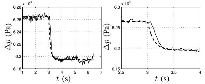
Fig. 7. Measured step response data (-) and model predictions (- -) at  $N = 9,432$  rpm,  $u_{s,0} = 0.409$ ,  $\delta u_s = 0.287$ . Whole time-span (left figure) and zoomed plot around  $t = 3$  s. (right figure).
