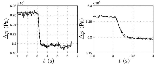
Fig. 8. Measured step response data (-) and model predictions with valve dynamics (- -) at  $N = 9,432$  rpm,  $u_{s,0} = 0.409$ ,  $\delta u_s = 0.287$ . Whole time-span (left figure) and zoomed plot around  $t = 3$  s. (right figure).
