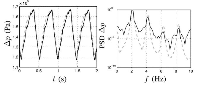
Fig. 5. Pressure difference and power spectral density of surge measurement (-) and simulation (- -) at  $N = 11,284$  rpm. Model parameter  $L_c$  increased by 100 % and  $\Delta p_c(0)$  increased by 2.5 % for this simulation.
