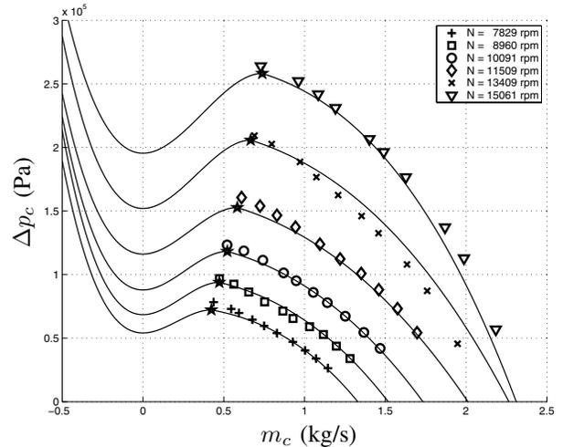
Fig. 3. Steady-state compressor map  $\Delta p_c(m_c, N)$  with measured operating points and points on the approximated surge line (\*).
