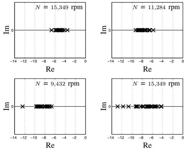
Fig. 11. Pole locations of the LTI approximations for all step response measurements at different operating conditions. Results in lower right figure obtained with  $u_{s,0} = 0.409$ ,  $\delta u_s = 0.172$ .
