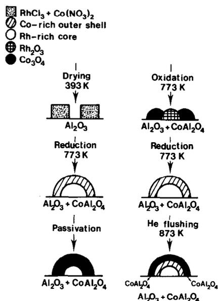
Fig. 6. Formation of bimetallic  $\text{CoRh}$  particles during reduction of the impregnated catalyst and the change in structure of the particles after different treatments.
