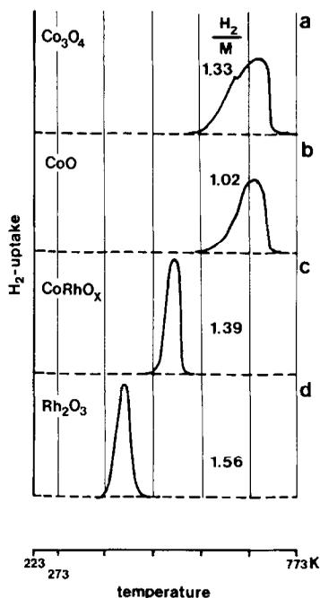
FIG. 3. TPR profiles for bulk oxides. (a) Co<sub>3</sub>O<sub>4</sub>, (b) CoO, (c) CoRhO<sub>x</sub>, and (d) Rh<sub>2</sub>O<sub>3</sub>.
