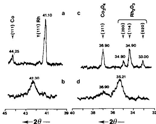
FIG. 2. X-Ray diffraction patterns (CuK $\alpha$  radiation). (a) Physical mixture of metallic Co and Rh, (b) Co-Rh alloy (molar ratio is 1), (c) physical mixture of Co<sub>3</sub>O<sub>4</sub> and Rh<sub>2</sub>O<sub>3</sub>, (d) CoRhO<sub>x</sub> mixed oxide.
