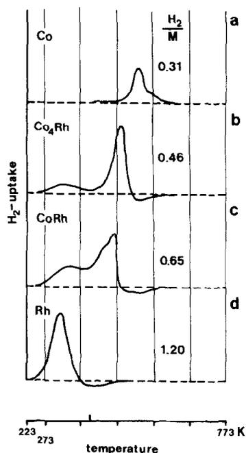
FIG. 5. TPR profiles for passivated alumina-supported catalysts. (a) Co (4.44 wt%), (b) Co<sub>4</sub>Rh (4.57 wt%), (c) CoRh (5.40 wt%), and (d) Rh (2.30 wt%) catalysts.
