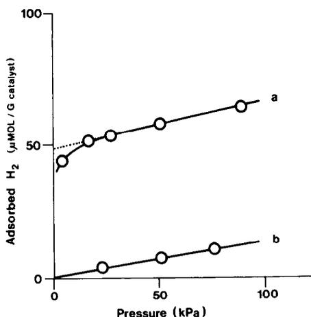
FIG. 1. Hydrogen chemisorption isotherms measured at 298 K for the 0.57 wt% Rh/Al<sub>2</sub>O<sub>3</sub> catalyst. (a) Catalyst, (b) bare support.
