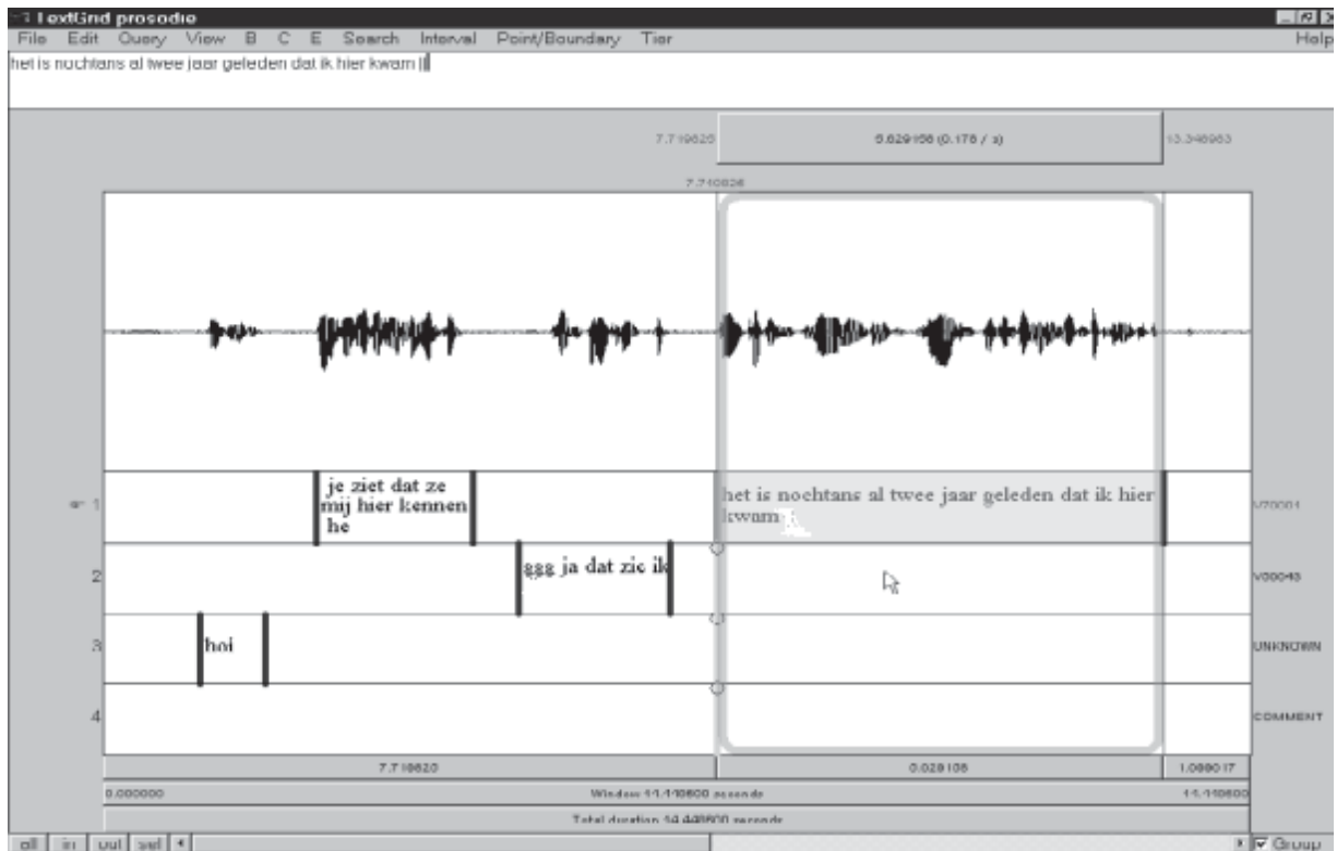
Figure 1. Sample screen of the Praat user interface. A single waveform is shown in the top window. Interactants are represented on separate text tiers (speaker 1, speaker 2, unknown third speaker). Vertical black bars indicate automatically detected strong phrase boundaries (see text).
