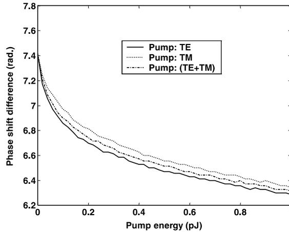
Fig. 6. Net phase shift difference  $\Delta\phi$  between TE and TM modes ( $\Delta\phi = \phi^{\text{TE}} - \phi^{\text{TM}}$ ) as function of pump pulse energy, where probe pulse polarizations are the same as Fig. 1.
