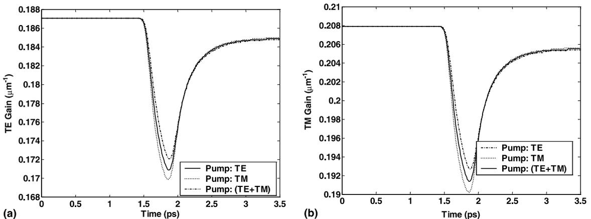
Fig. 3. Time variation of gain at the middle of SOA (at  $125 \mu\text{m}$ ), where the pump pulse energies are 0.5 pJ, and the pump pulse polarizations are the same as Fig. 1. In (a) the TE gain and in (b) the TM gain are shown.
