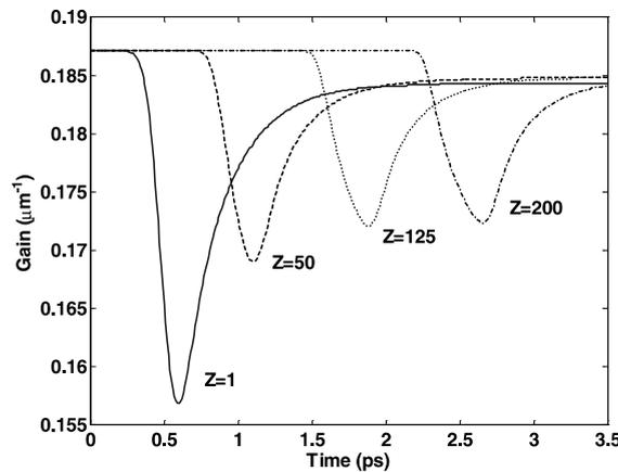
Fig. 2. Time variation of gain at different positions  $z$  (in  $\mu\text{m}$ ) of the SOA, where the input pulse energies are 1 pJ with TE mode.
