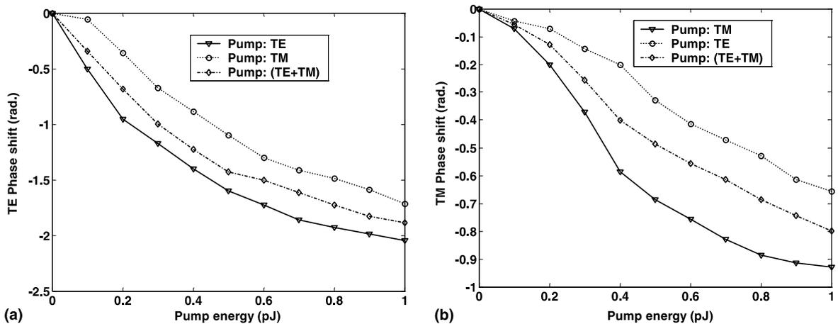
Fig. 5. Phase shifts of the 0.4 fJ, 200 fs probe pulse as function of pump pulse energies under the same conditions as in Fig. 4. In (a) the phase shift of TE component of probe pulse and in (b) the TM component of probe pulse are shown.
