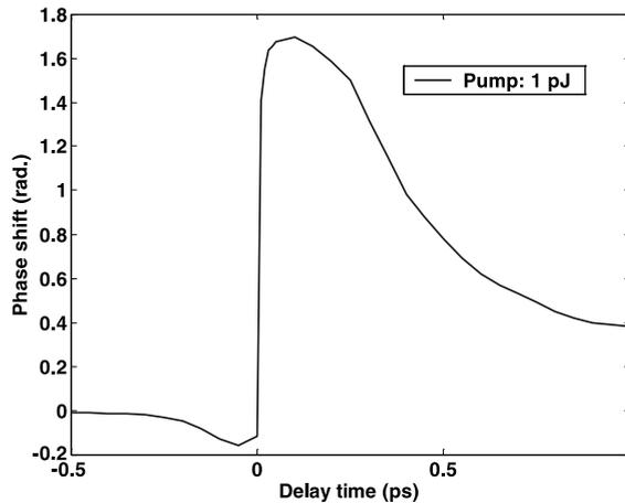
Fig. 7. Phase modulation of the probe pulse as function of pump–probe pulse delay time, where both of the probe and pump pulse are TE polarized.
