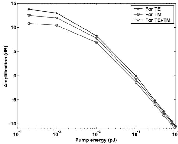
Fig. 1. Net amplification of the SOA as a function of the pump pulse energy, where the pulse width is 200 fs, and the pump is linearly polarized along the TE, the TM polarization axis or 45° with respect to the polarization axes of TE and TM modes (noted as TE + TM).
