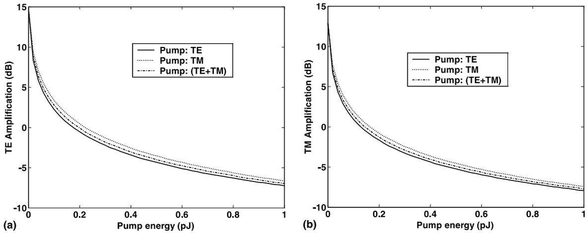
Fig. 4. Net amplification of the 0.4 fJ, 200 fs probe pulse as a function of the pump pulse energy, where the pump pulse polarizations are the same as Fig. 1. In (a), the TE amplification and in (b), the TM amplification are shown.
