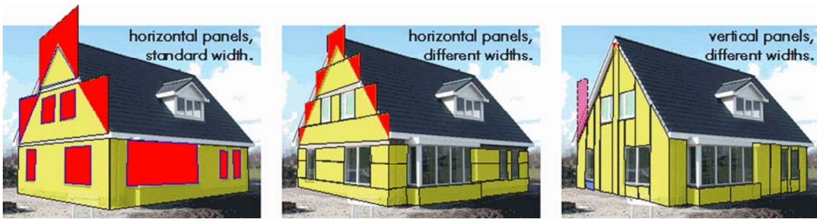
Figure 1: Feasible set-ups for full industrially produced walls. Set-up right is adopted in this study.
