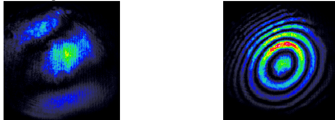
Figure 6. Interference patterns recorded from the Michelson interferometer for (a) all the actuators were set at 0V, and (b) all actuators set to 200V.
