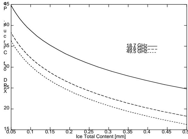
Figure 2.4-5: Crosspolar discrimination (XPD) for circular polarisation at Ka and V-Band, versus total ice content. The ice needles are aligned. Rotation angle,  $\gamma = 90^\circ$ . Link elevation =  $41^\circ$
