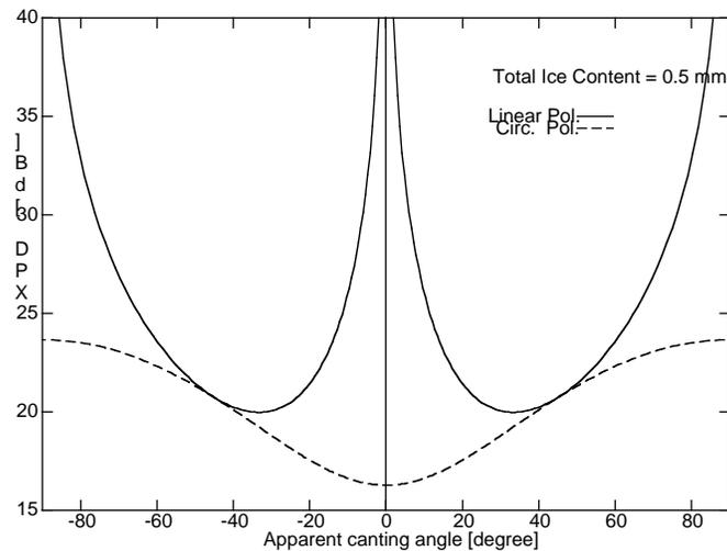
Figure 2.4-6: Cross-Polar Discrimination of linear and circular polarisations due to ice, as a function of the apparent canting angle of the ice cloud, at 50 GHz. The total ice content is 0.5 mm. The link elevation is  $41^\circ$
