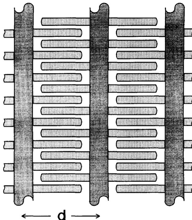
Figure 1 Schematic representation of the layered mesophase; the main chains are separated by the interdigitating side chains at the layer distance  $d$  (after Ballauff<sup>10</sup>)
