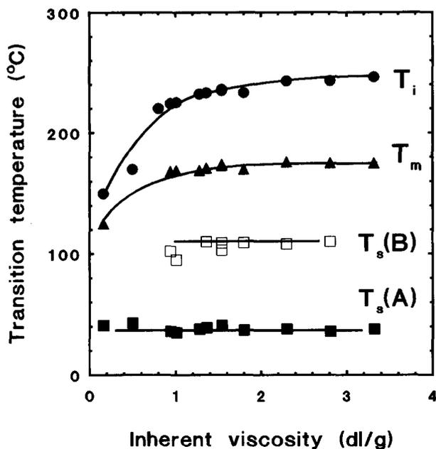
**Figure 4** Transition temperatures  $T_s(A)$  (■),  $T_m$  (▲) and  $T_i$  (●) (all from the second heating runs) and  $T_s(B)$  (□) (from the first heating run) as functions of the inherent viscosity for PTA12HQ. Data below  $\eta_{inh} = 0.6 \text{ dl g}^{-1}$  were taken from Ballauff<sup>7</sup>
