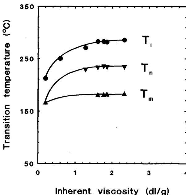
**Figure 6** Transition temperatures  $T_m$  (▲),  $T_n$  (▼) and  $T_i$  (●) as functions of the inherent viscosity for PTA6HQ (from first heating runs). Data below  $\eta_{inh} = 1.4 \text{ dl g}^{-1}$  were taken from Ballauff<sup>7</sup> and Falk<sup>11</sup>
