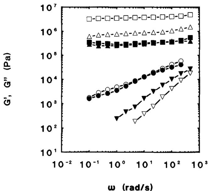
Figure 10 Storage and loss moduli of PTA6HQ in the solid phase ( $\square$ ,  $\blacksquare$ , 150°C), the layered mesophase ( $\triangle$ ,  $\blacktriangle$ , 200°C), the nematic mesophase ( $\nabla$ ,  $\blacktriangledown$ , 250°C) and the isotropic phase ( $\circ$ ,  $\bullet$ , 295°C). Open symbols refer to the storage modulus  $G'$ , closed symbols to the loss modulus  $G''$
