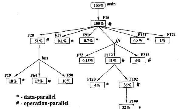
Figure 7: Context graph for the frequency tracking system
