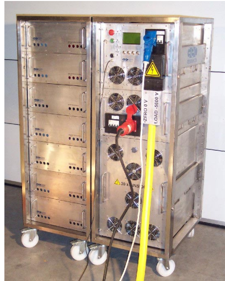
Fig.3. All solid-state switch pulsed power source (courtesy of Geo-Resource, B.V., Rotterdam, The Netherlands).
