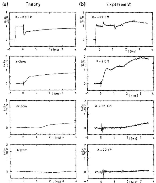
FIG. 3. Response of a porous medium to a stepwise pressure wave at normal incidence. Air volume fraction in pores  $(2.3 \pm 0.2) \cdot 10^{-3}$ , mean bubble radius: 0.8 mm. Pressure time histories above the column ( $-89 \text{ cm}$ ), and at distances 2, 12, and 22 cm from the surface inside the column.
