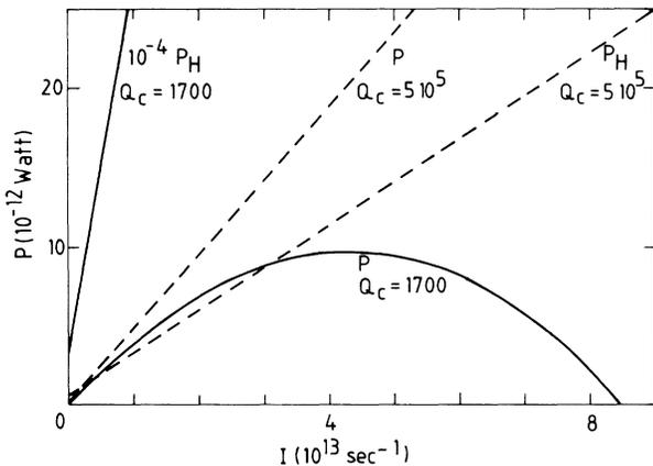
FIG. 2. Power  $P$  vs surplus flux, compared to threshold power  $P_H$  for onset of nonsteady oscillation. Solid lines: actual parameter values for the University of British Columbia maser. Dashed lines: increased  $Q_c$  value.
