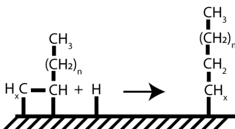
Figure 2.2: Schematic view of the hydrogenation reaction on the second carbon in the growing hydrocarbon chain.
