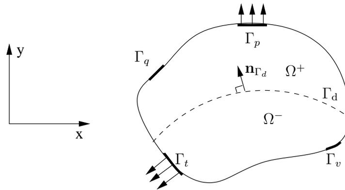
**Figure 1.** Body  $\Omega$  crossed by a discontinuity  $\Gamma_d$  and complemented by boundary conditions. The x-y coordinate represents the global coordinate of the body.
