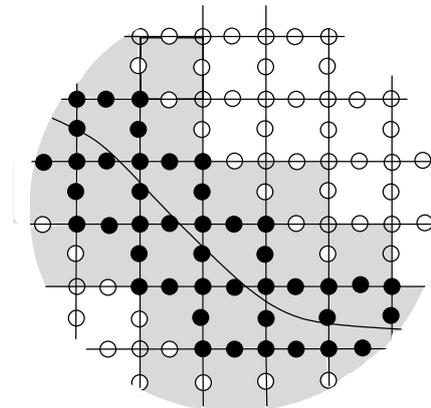
**Figure 4.** Two-dimensional finite element mesh with a discontinuity denoted by the bold line. Nodes with enhanced degrees of freedom are indicated by solid dots. The grey elements contain additional terms in the stiffness matrix and the internal force vector.
