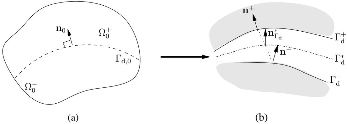
**Figure 2.** (a). Schematic representation of body  $\Omega_0$  crossed by a material discontinuity  $\Gamma_{d,0}$  in the undeformed configuration. (b). Discontinuity interfaces  $\Gamma_d^+$  and  $\Gamma_d^-$  and their normal vector representation in the deformed configuration
