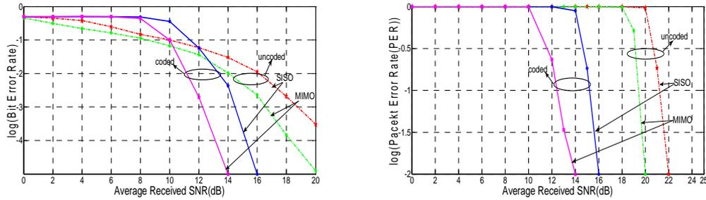
**Fig. 4:** BER and PER performance of multiband OFDM with various diversity orders.
