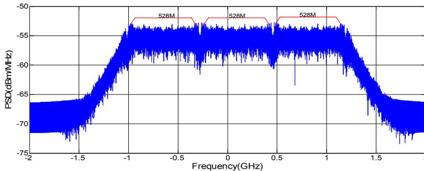
**Fig. 2:** Transmission of MB-OFDM UWB signal
