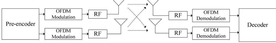
**Fig. 3:** MIMO-OFDM communication system
