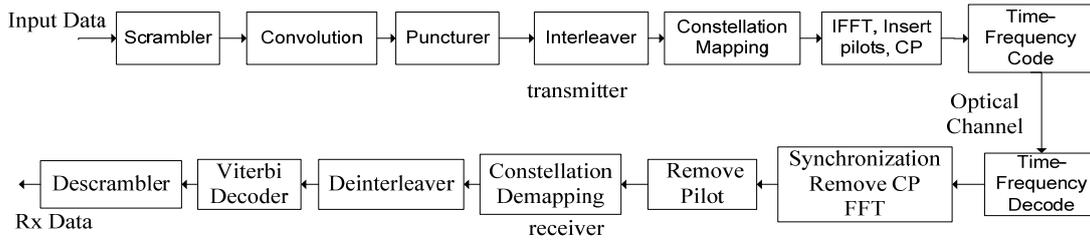
**Fig. 1:** Multiband OFDM transmission system
