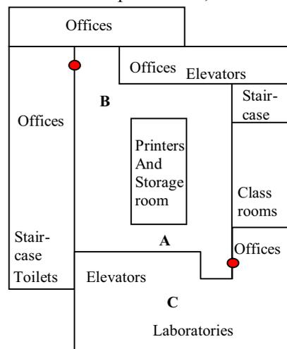
Fig. 8 Simplified floor plan of the 13<sup>th</sup> floor of the building housing the Faculty of Electrical Engineering of Eindhoven University of Technology. Red dots indicate the positions of the WLAN routers. Measurement positions are A (distance to router: 7.05m), B (distance to router: 8.05m) and C (distance to router: 12.30m).
