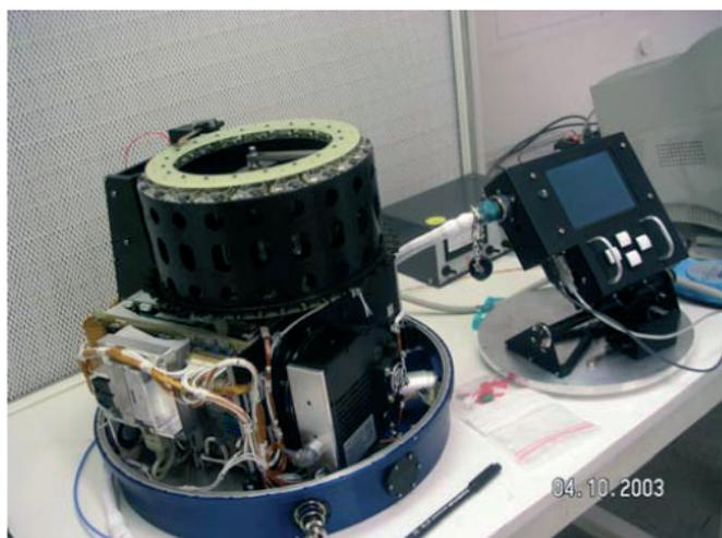
Figure 4: The interior of the Arges container, together with the HMI, prior to closure of the container with the aluminium dome.
