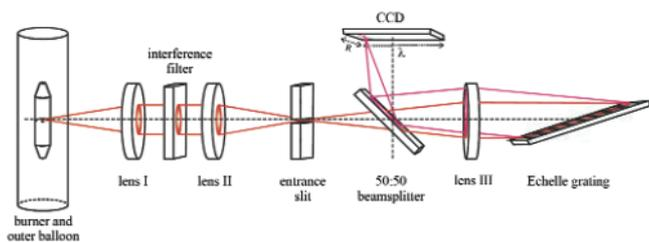
Figure 2: Schematic view of the integrated emission spectrometer. An Echelle type spectrometer is used in the Littrow configuration, meaning that the imaging lens (III) is used for the collimation of both the undispersed beam of light as well as the reflected dispersed beam of light.
