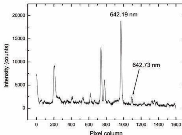
Figure 6: Measured spectrum of a Dy lamp at a certain lateral position during microgravity phase.
