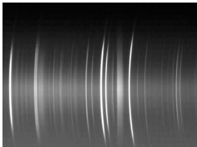
Figure 3: Example of a 2-D image as it is recorded by the integrated CCD camera. The horizontal axis represents the wavelength, the vertical axis the lateral position in the burner. The spectral lines appear to be curved. This is, however, an artefact which results from peculiarities in the diffraction at the Echelle grating. Ex posteriori the images are processed to straighten the lines.
