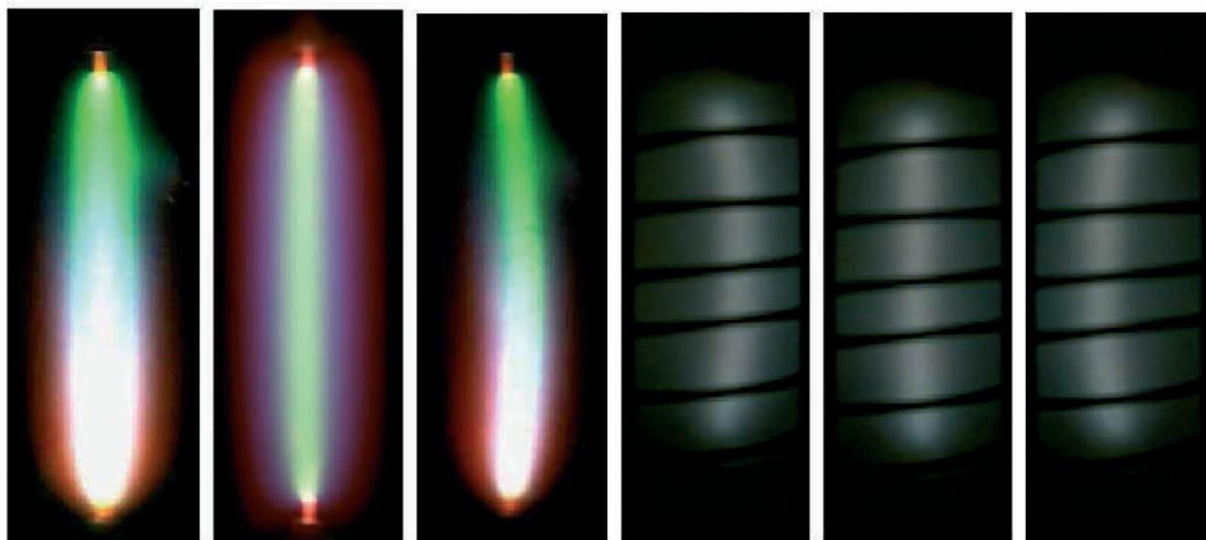
Figure 8: pictures of the plasma in the lamp. (a): on the ground, axial demixing is vlearly visible; (b): same lamp in space: only radial demixing is observed, no axial demixing; (c): helical instability on the ground; (d), (e) and (f): helical instability in space, with suppressed axial demixing and with very slow rotation due to residual gravity of 0.001 g.
