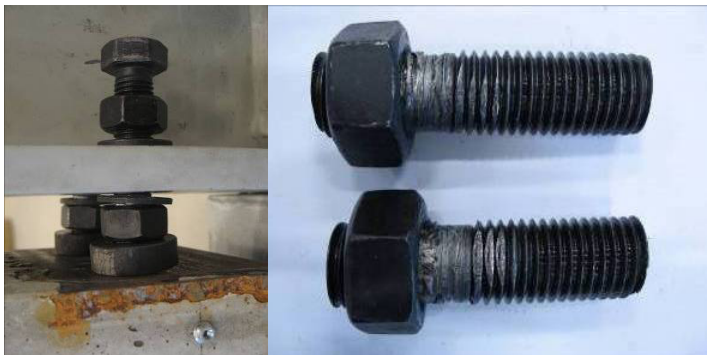
Fig. 6: Failure of discrete steel-concrete connection by bolt shear through nut
