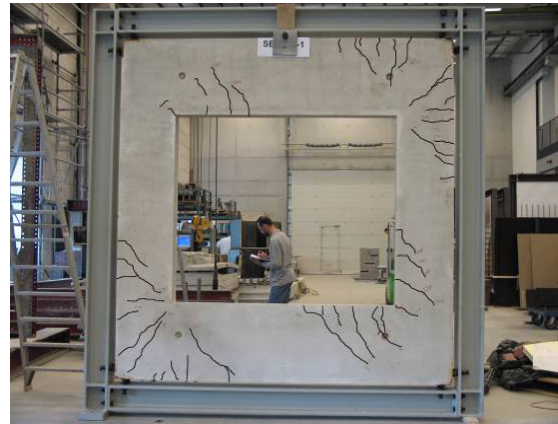
Fig. 13: Smeared crack pattern versus experimental crack pattern (specimen 3)
