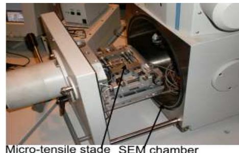
Figure 2: Micro-tensile stage in scanning electron microscope chamber.
