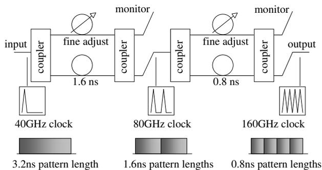
Fig. 9. Experimental arrangement for generating pseudo random bit sequences at  $2^7-1$  at 160Gb/s using optical time division multiplexing. This apparatus is an explicit description of the functional block shown as x4 in figure 5.
