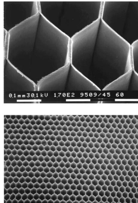
**Figure 3.** Scanning electron micrographs of a foil-based honeycomb made of polyester foil with a thickness of  $5\ \mu\text{m}$  covered by 20 nm Al. The width of the foil-to-foil joints is  $150\ \mu\text{m}$ .
