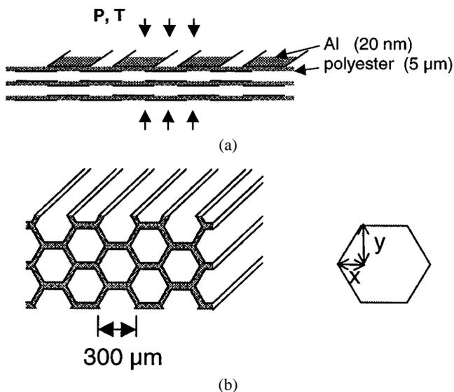
**Figure 1.** Fabrication of a foil-based multichannel structure. (a) Stacking of polyester foils with a patterned Al coating. The foil-to-foil joints are established by the application of elevated temperature and high pressure. (b) Resulting honeycomb structure after expansion of the foil stack. The  $x$ - $y$  coordinates for the deformation model are shown.
