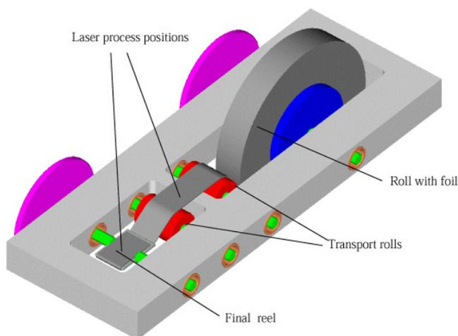
**Figure 2.** Schematic diagram of the reel-to-reel foil processing tool.
