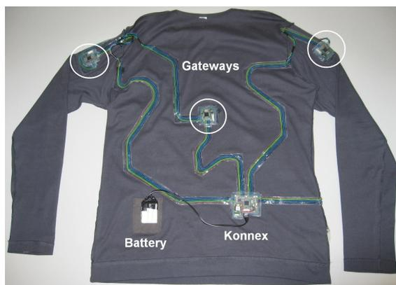
Fig. 1. SMASH system (inner side) with the Konnex and three Gateways (marked with a circle). The fourth Gateway is hidden.
