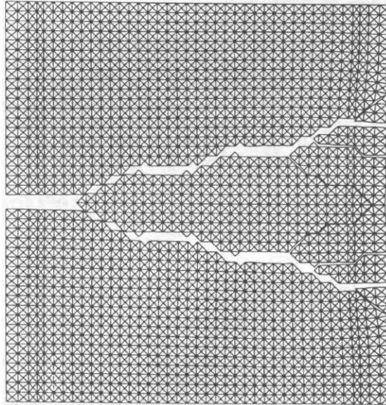
Figure 1: Simulation of crack branching in Polymethyl Methacrylate (PMMA) using inter-element cohesive surface models [12]. Note that although the crack can only propagate in the  $0^\circ$ ,  $\pm 45^\circ$  and  $90^\circ$  directions, the propagation in other directions is captured relatively well.
