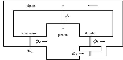
Figure 2: Lumped parameter compression system model.
