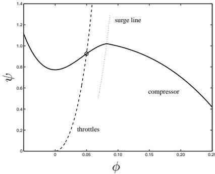
Figure 1: Compressor curve with unstable operating point.
