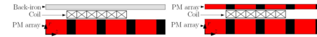
Figure 1 Moving coil TPMA with (a) soft magnetic back iron (b) double sided magnet array
