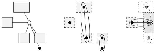
**Figure 12:** Abuttability of pins (left) is translated into an *Abuttability Graph* (center). A *Maximum Matching* algorithm selects edges, yielding a side assignment. In a next step, pins can also be abutted against *wires* created for a selected edge in the previous step (right).
