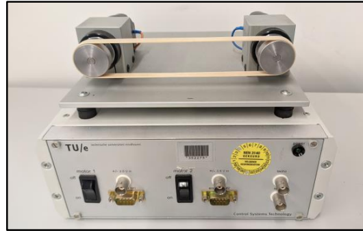
Figure 4: Experimental setup used for validating the developed framework. It consists of two rotating masses connected via a rubber band. The masses are both actuated by a DC motor. The right mass is virtually suspended to the fixed world by feedback control.
