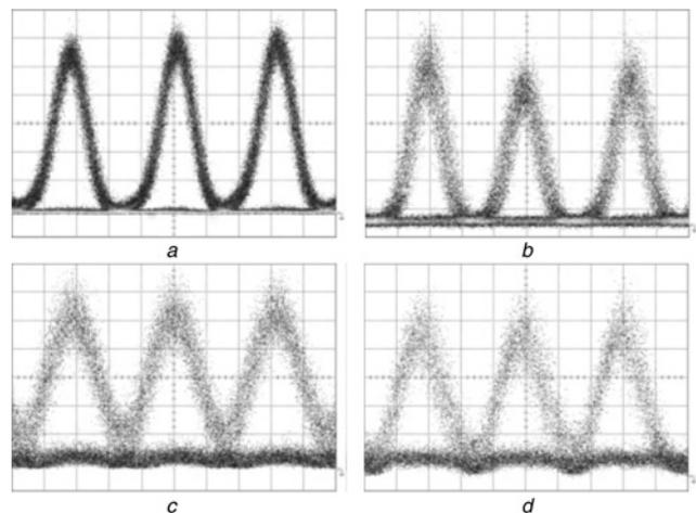
**Fig. 2** Eye diagrams of 160 Gbit/s signal across system (2 ps/div.)
