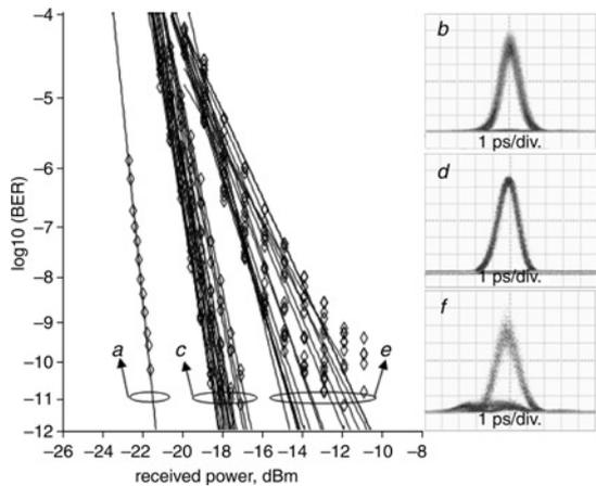
**Fig. 3** BER curves and associated demultiplexed eye diagrams of: 10 Gbit/s original channel (Figs. 3a, b), back-to-back situation (Figs. 3c, d), and transmission through the whole two 50 km fibre links (Figs. 3e, f)
