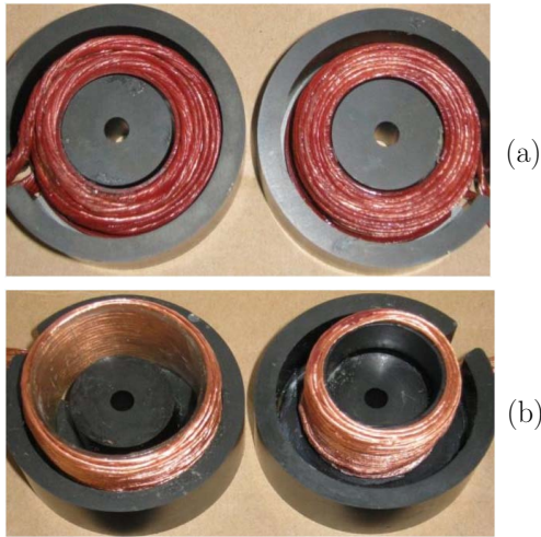
Fig. 13. Manufactured transformers (a) adjacent winding topology and (b) coaxial winding topology.
