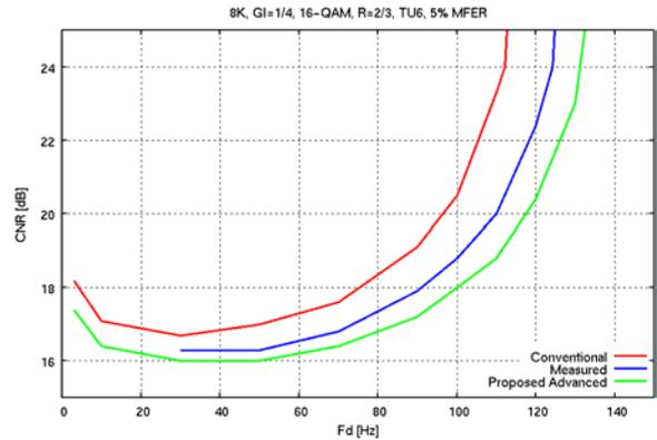
Fig. 3. Measured 5% MFER performance for a TU6 channel.
