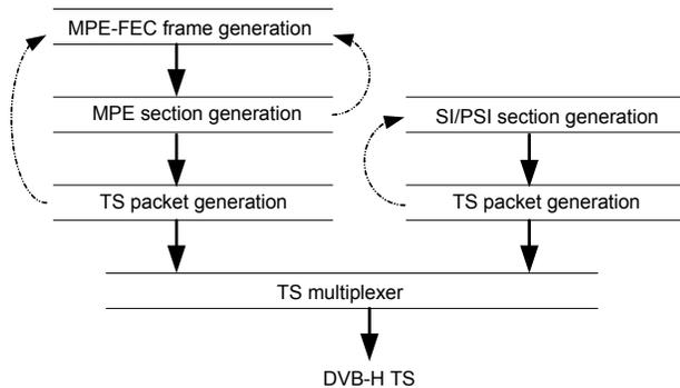
Fig. 2. DVB-H generator, with at the left side the IP-flow and at the right side, the SI/PSI flow. The generators at the top also generate the reference data. Via back annotation, dashed lines, the generators are informed of errors on purposely inserted during encapsulation resulting in an MPE-FEC frame equipped with erasure information or absence of SI/PSI sections in the reference set.
