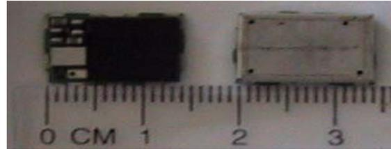
Fig. 1. At the right side an unshielded and at the left side the shielded version of a DVB-H receiver.
