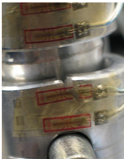
Figure 13. Structural failure due to extended cracking at the centre point
