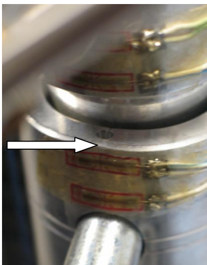
Figure 12. Start of crack at the centre point
