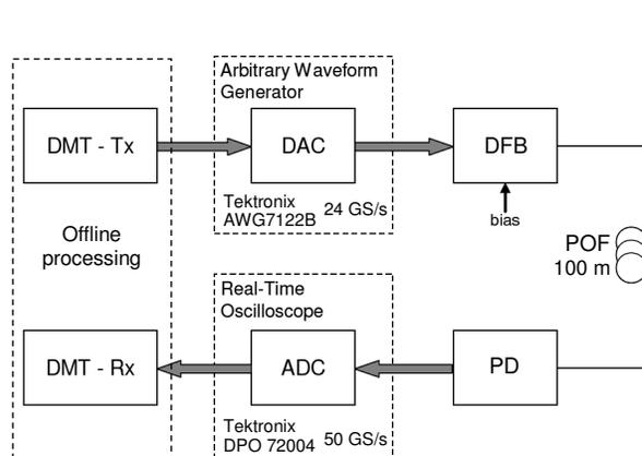
Fig. 1. Measurement setup for DMT over POF transmission
