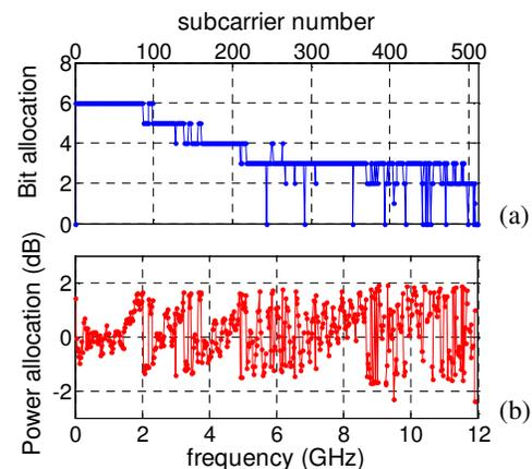
Fig. 2(a) Bit allocation map for 40 Gb/s bit rate; (b) Power allocation for 40Gb/s bit rate
