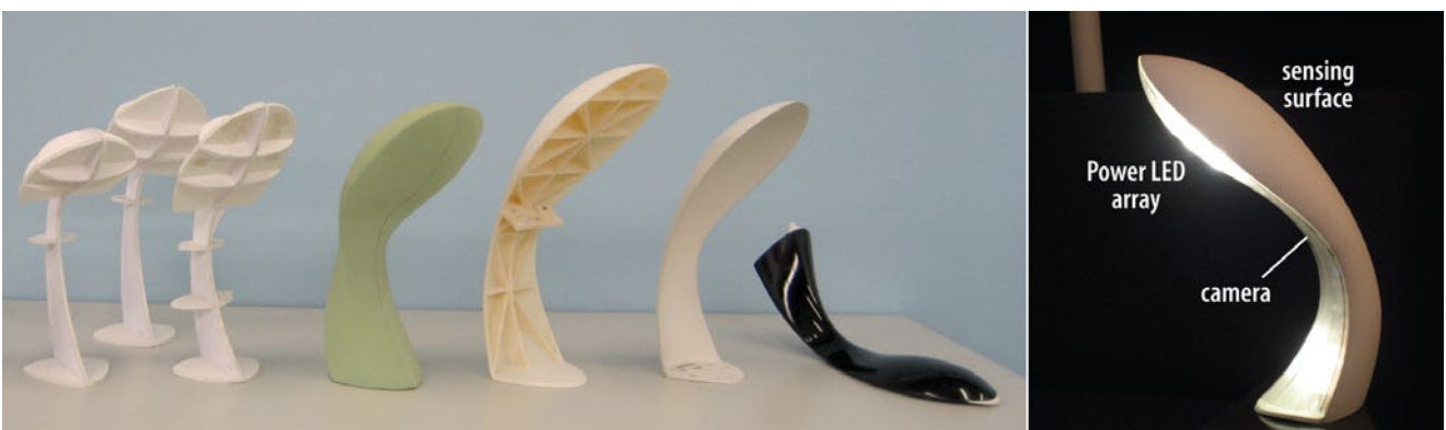
Figure 7. Left picture: Consecutive stages of the final lamp body design. The lamp body developed into an organic physical shape to invite and suit hand gestures on its surface. Much attention was given to the definition of the shape and its material. Right picture: The lamp body with its sensory-motor system. Its form was designed to be neutral, but versatile enough to be able to portray all three behaviors specified in the criteria. A touch sensitive area and a Power LED matrix were implemented at the back and front of the lamp respectively. The lamp also had a camera that allowed it to detect the position of nearby reading material.
