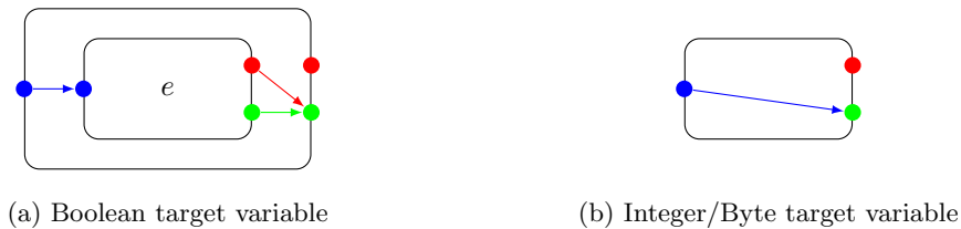
Figure 5.5: The patterns used to construct an atomic node for an assignment object.
