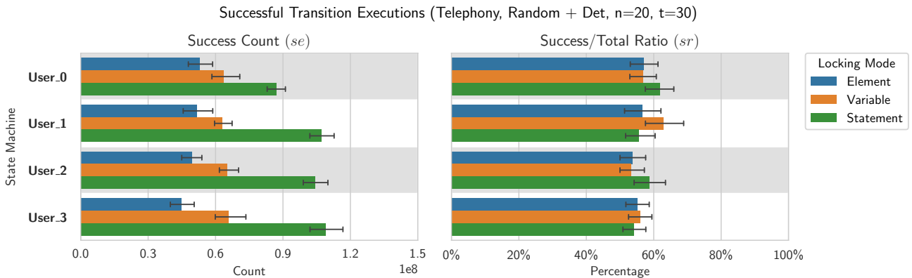
Figure 8.17: A bar plot that reports the number of successful executions ( se ) and the percentage of successful executions ( sr ) for each state machine in the target model Telephony , where the results are grouped by the locking mode. The results have been measured over a time span of 30 seconds, where each entry is represented by measurements taken over 20 trials.
