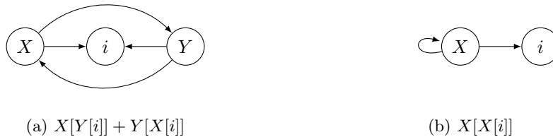
Figure 5.2: Graph visualizations of inter-lock-dependencies for several statements. In this figure, the indices that accompany the variables have been obfuscated due to them being superfluous.
